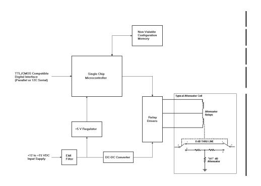
Figure 1. SmartStep Driver Circuitry
